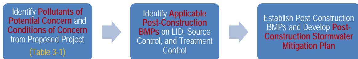
Figure 3-1 Post-Construction BMP Selection Procedure Flow Chart
