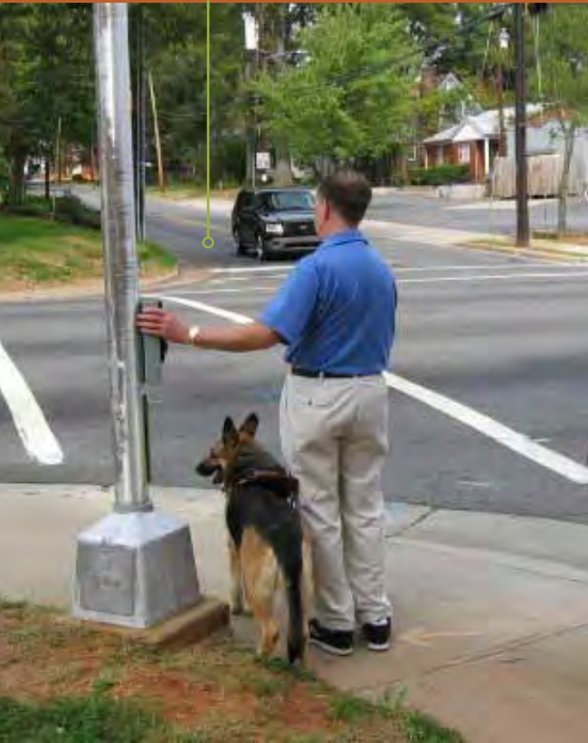
A pedestrian waits to feel the vibrotactile walk signal at an intersection. (NCHRP)
