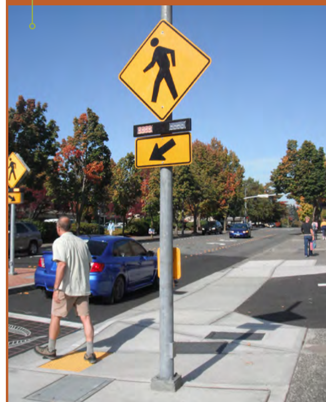
Flashing warning light (Rectangular Rapid Flash Beacon—RRFB)
