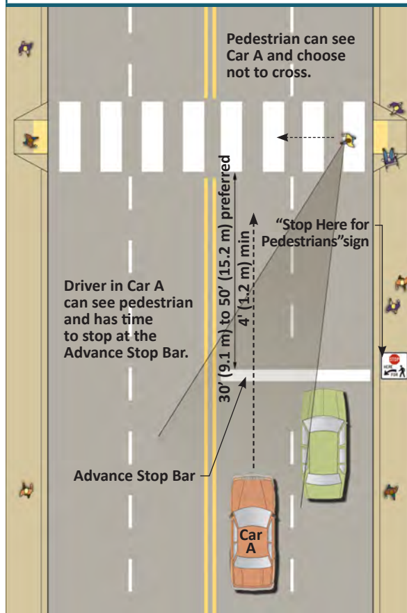
EXHIBIT 5.4 An advance stop bar gives both pedestrians and motorists better visibility.
