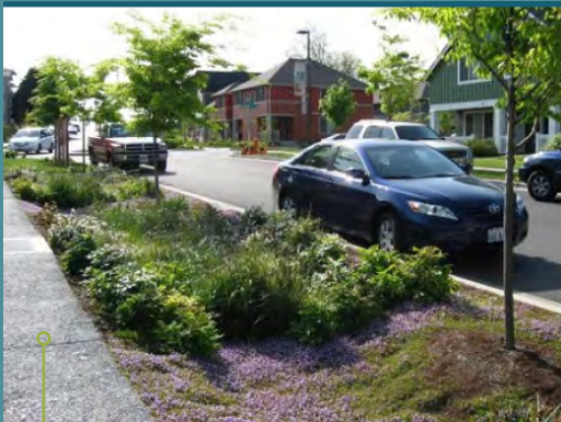
A bioswale was designed to convey and filter stormwater along this street in Seattle, WA. ( www.epa.gov )
