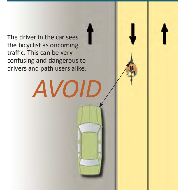
EXHIBIT 7.24 Avoid shared use paths directly adjacent to roadways unless buffer width can be provided.
