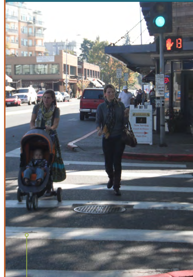
Pedestrian signal showing flashing upraised hand with countdown display, Kirkland, WA
