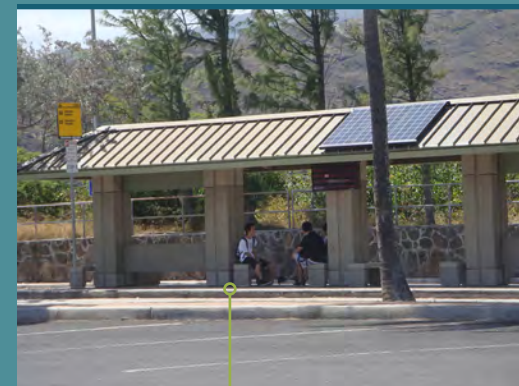
Transit shelter with photovoltaic system on roof
