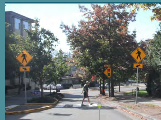
New mid-block crossing in a busy commercial area, designed with flashing signs and high contrast crossing area, Downtown Bellevue, WA
