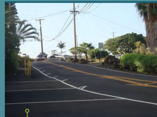
Shark's teeth markings help keep motorists on the roadway at difficult curves.
