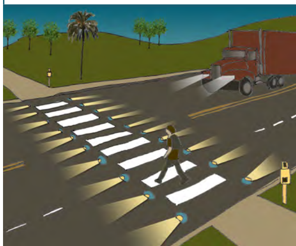
EXHIBIT 5.44 In-pavement warning lights make pedestrians more visible at night or in dark, cloudy conditions.
