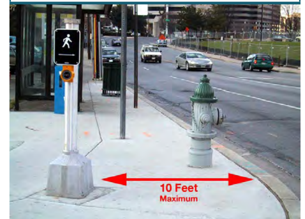
EXHIBIT 3.23 Push button must be within 10 feet of curb.
