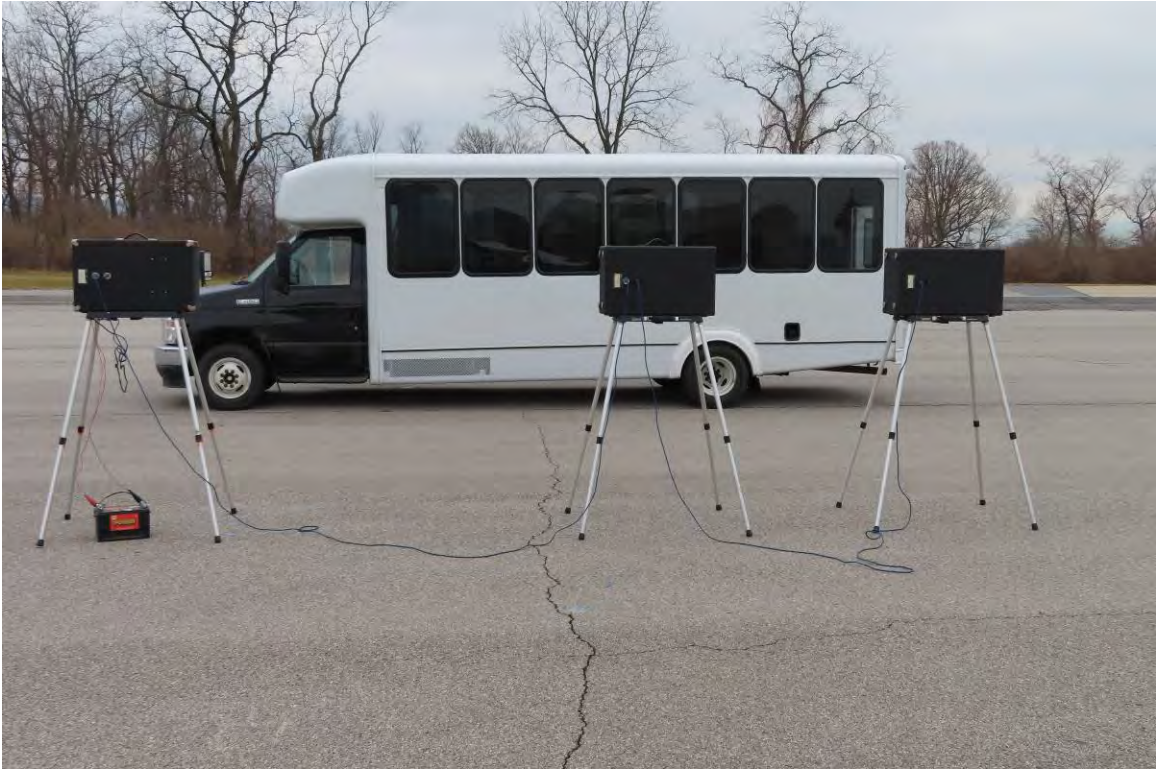
TEST BUS SET-UP FOR 80 dB(A) INTERIOR NOISE TEST
