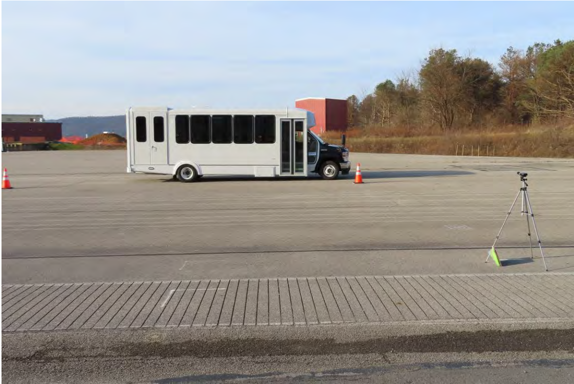
TEST BUS UNDERGOING EXTERIOR NOISE TESTING
