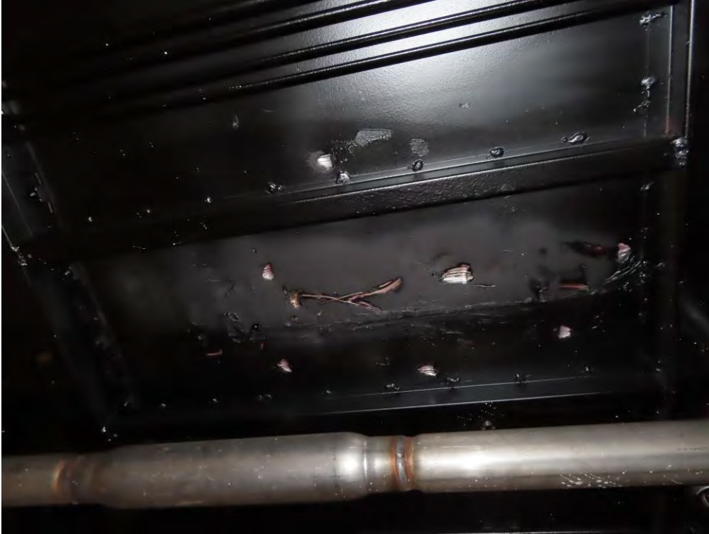
SCRAPES AND GOUGES ON UNDERSIDE OF BUS
