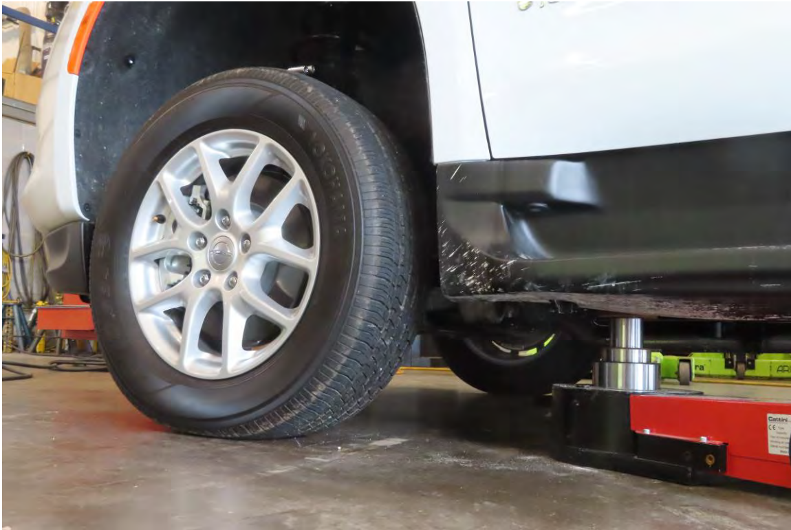
FRONT JACK IN PLACE
