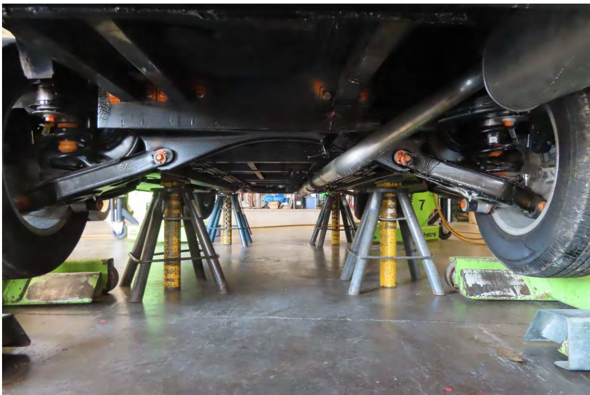
FRONT AND REAR JACK STANDS IN PLACE
