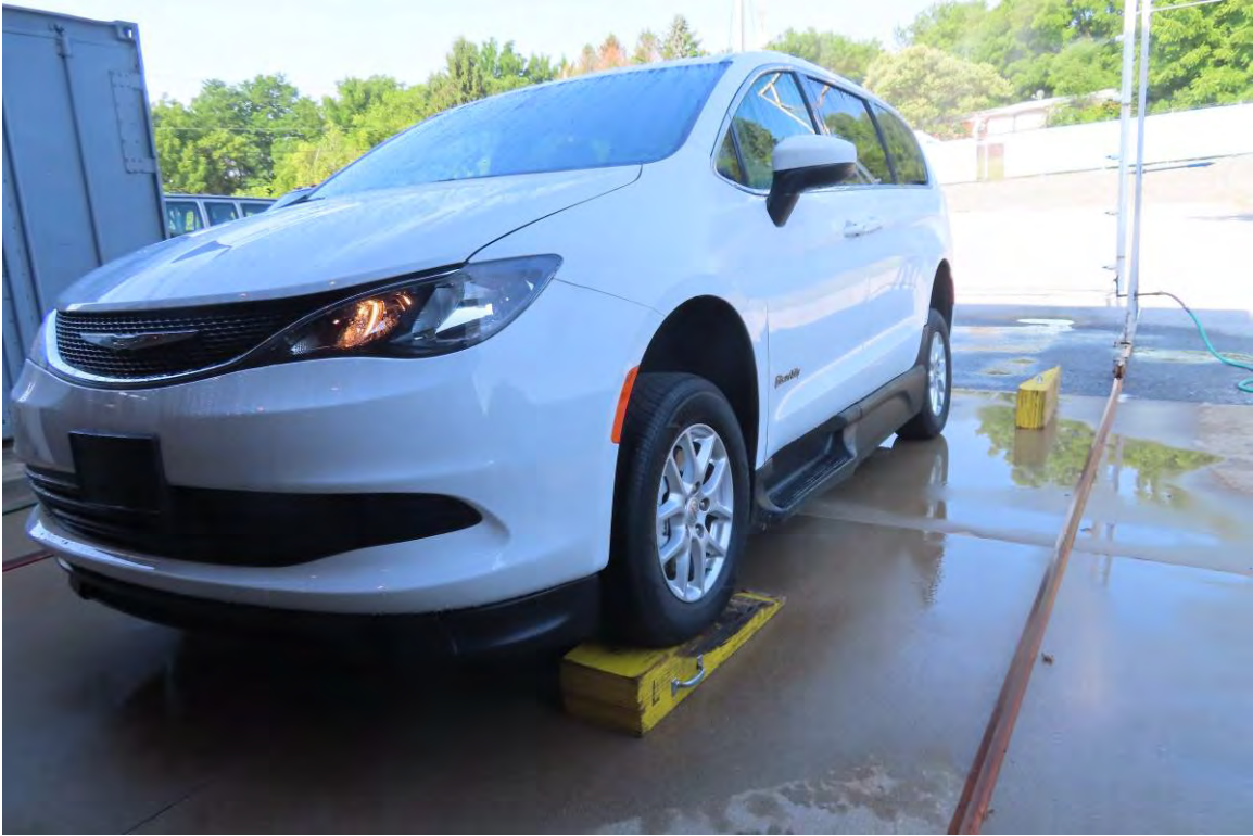
LEFT FRONT WHEEL SIX INCHES HIGHER
