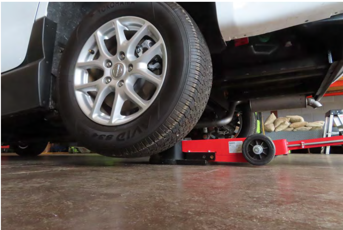
REAR JACK IN PLACE
