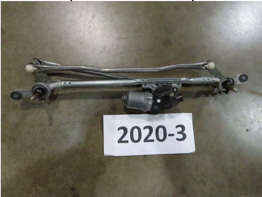
WIPER MOTOR REMOVAL AND REPLACEMENT (0.50 LABOR HOURS)
