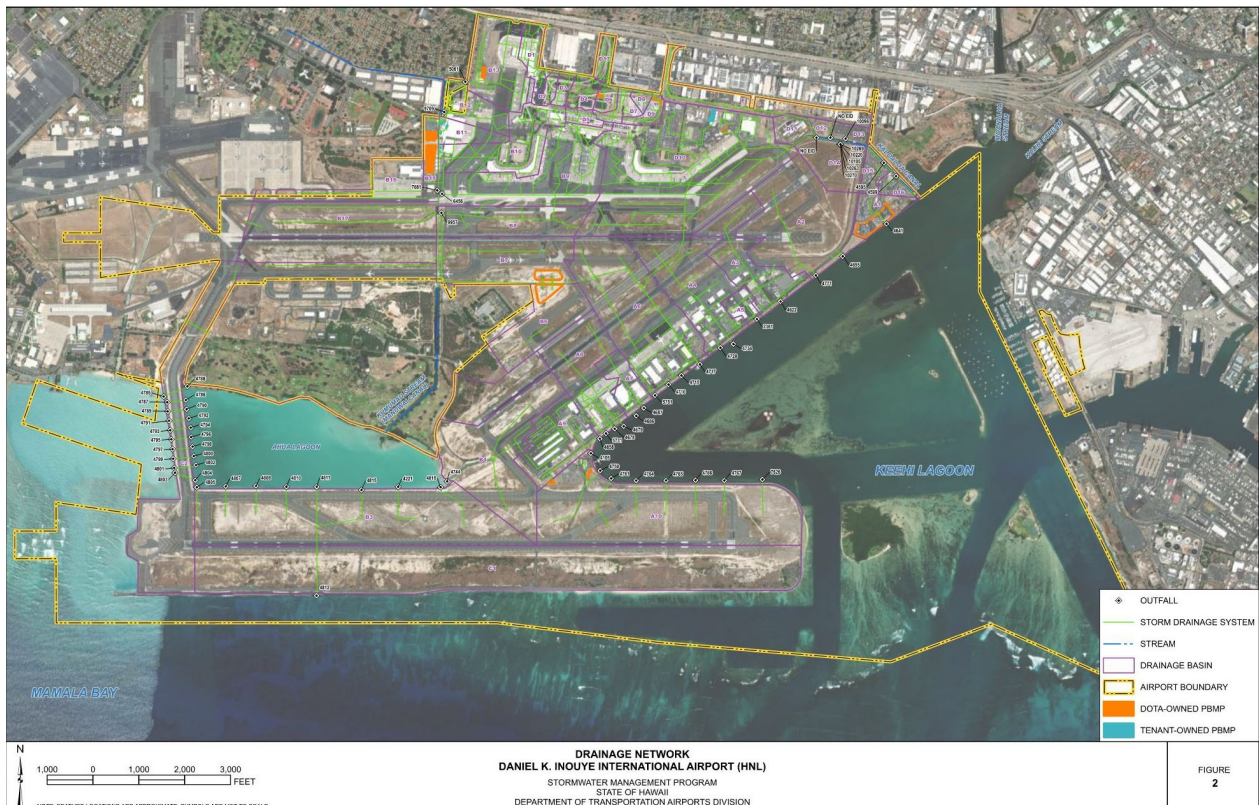
Figure 2: HNL Airport Boundary and Drainage Network.
