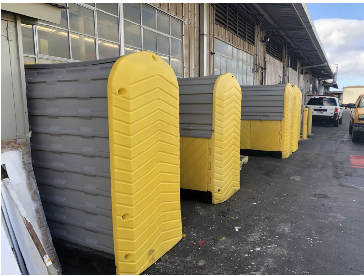
Photograph 30: Paint Storage area, with paint stored inside of the yellow clam shells.
