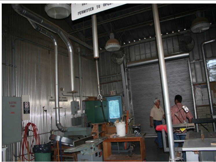
Photograph 24: Interior of the Carpentry Shop. Visible piping is a part of the sawdust vacuum system.
