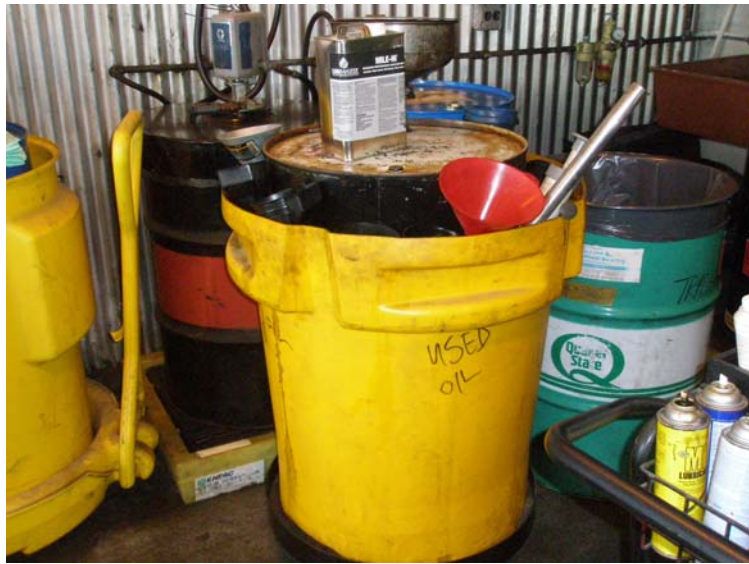
Photograph 7: 55-gallon drums of used oil in mobile over-pack containers.
