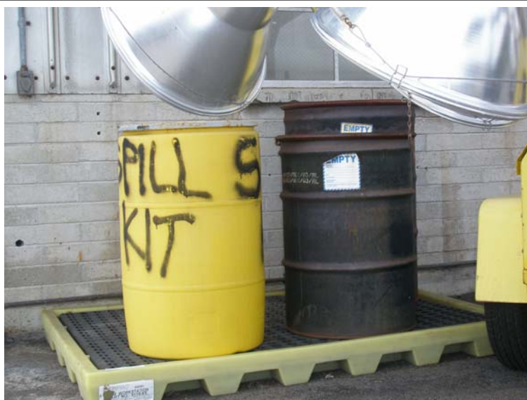
Photograph 9: Spill materials located outside of the maintenance shop near the fueling area.
