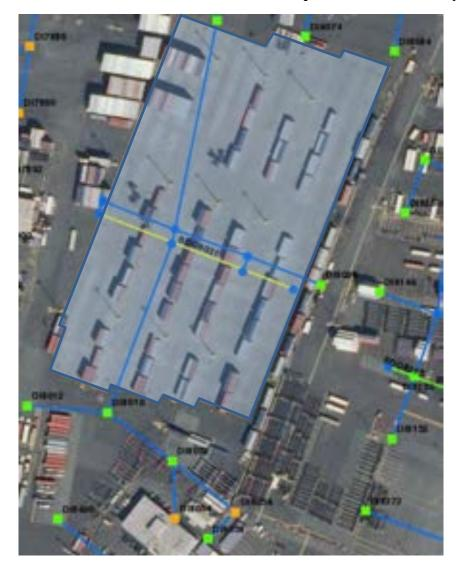
Figure 3-12 Pier 51B Container Yard Redevelopment Storm Sewer System
