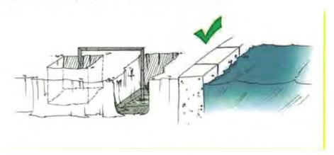
Upon acquisition of applicable government approval, contaminated water can be discharged into a newly excavated pit/trench within the impacted area.
