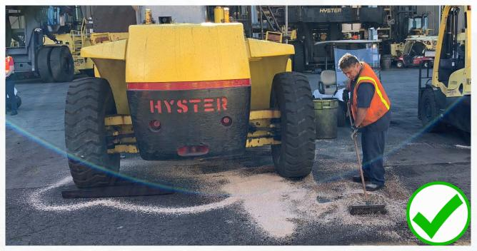
Contain the spill, stop the source, clean up and properly dispose of absorbent material
