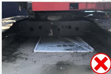
Utilizing a containment device, however the leak expands larger than the device
