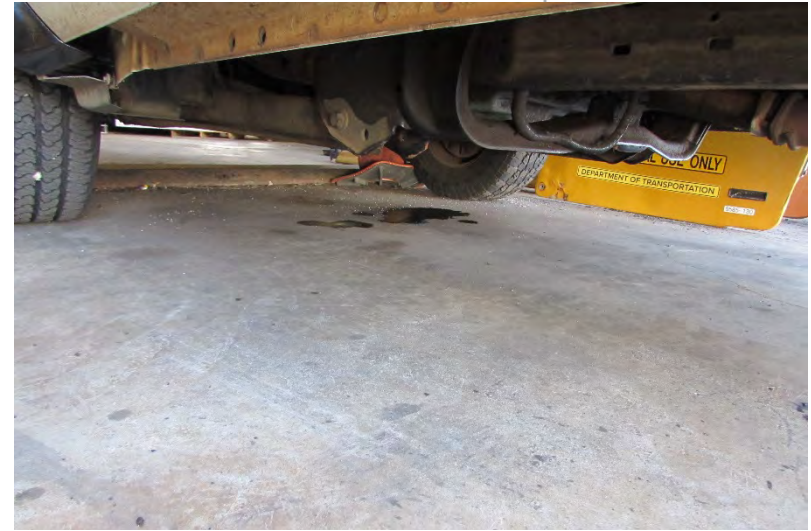
HWY-M Photo 5.2.98 Truck Storage Shed Oil Leak
