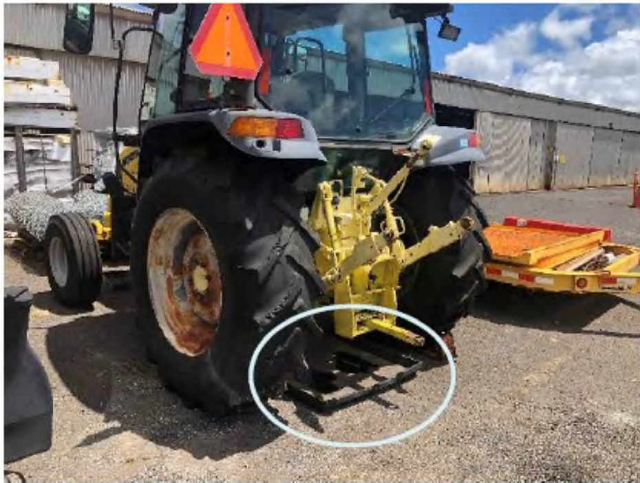
Figure 1. Drip pan placed underneath the leaking equipment.
