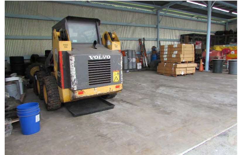
HWY-O Photo 6.2.58 Drip Pan Under Parked Equipment (in Vehicle Shed)
