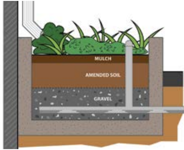
Figure 4.7: Schematic of Planter Box with Down Spout Connection and Underdrain
