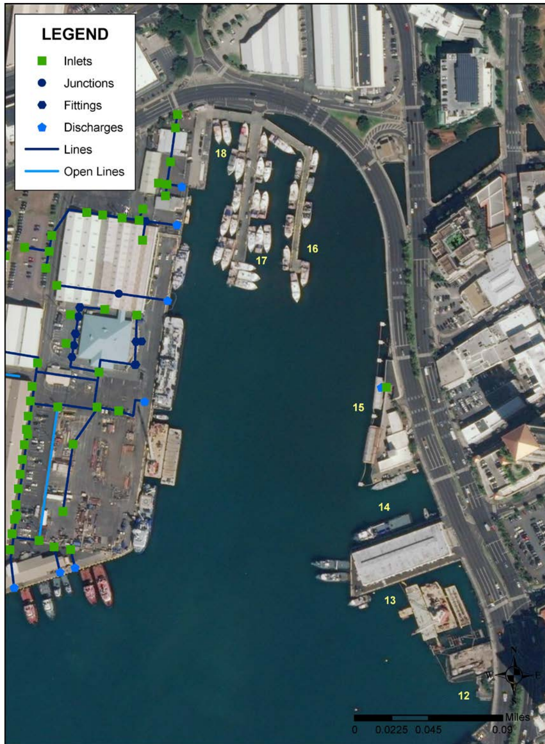
Figure 6. Piers 12 through 18 GIS map of storm drain assets.
