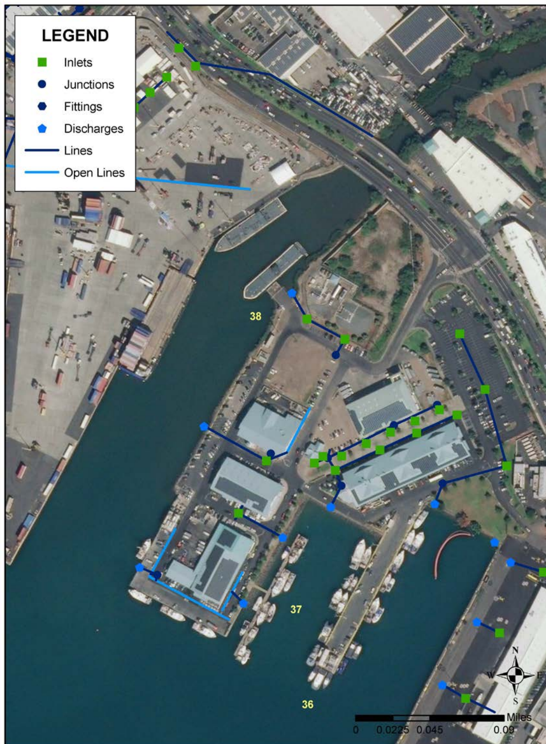
Figure 9. Piers 36 through 38 GIS map of storm drain assets.
