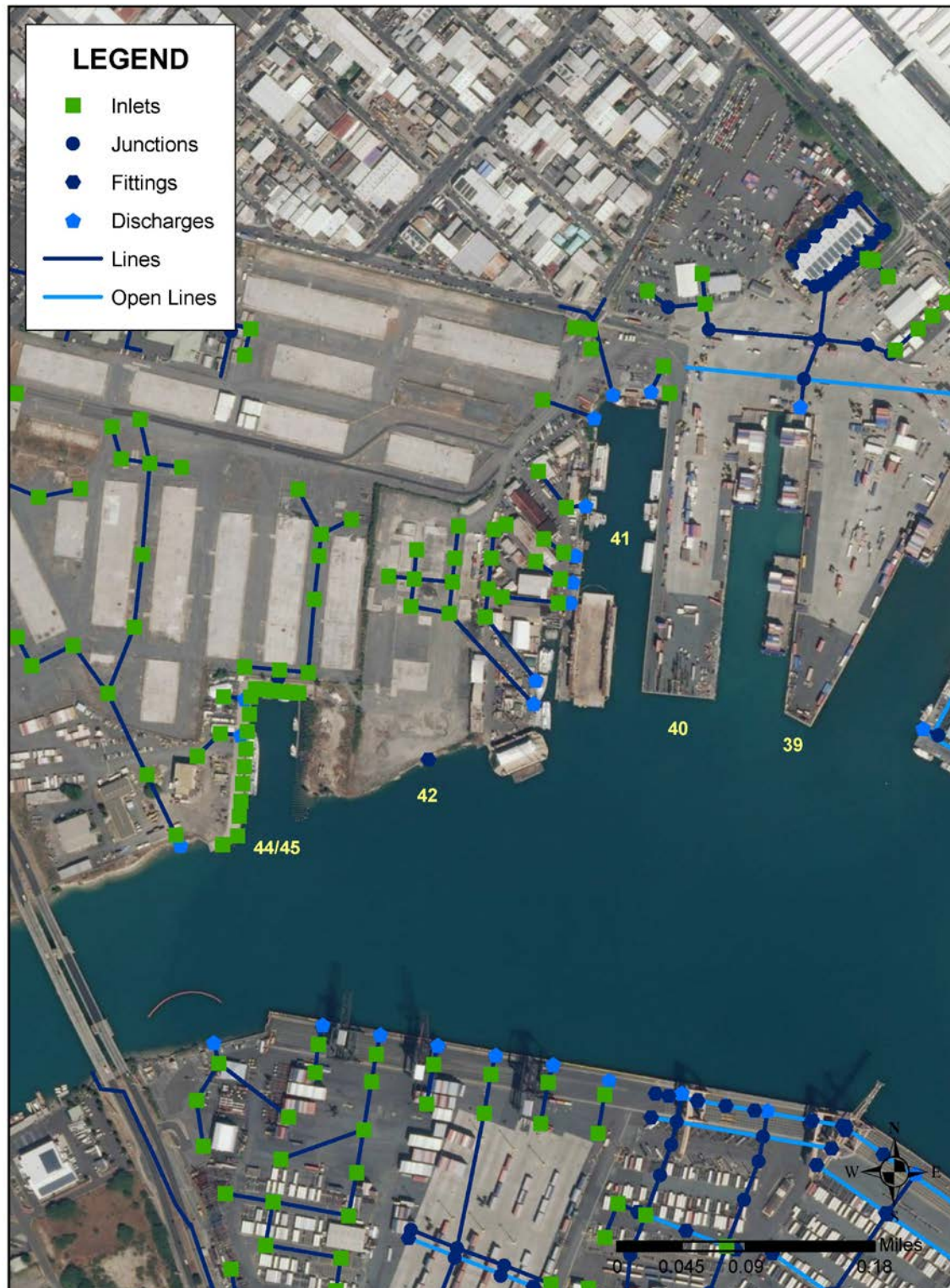
Figure 10. Piers 39 through 45 GIS map of storm drain assets.
