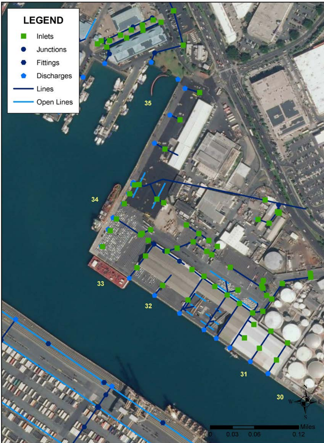
Figure 8. Piers 31 through 35 GIS map of storm drain assets.
