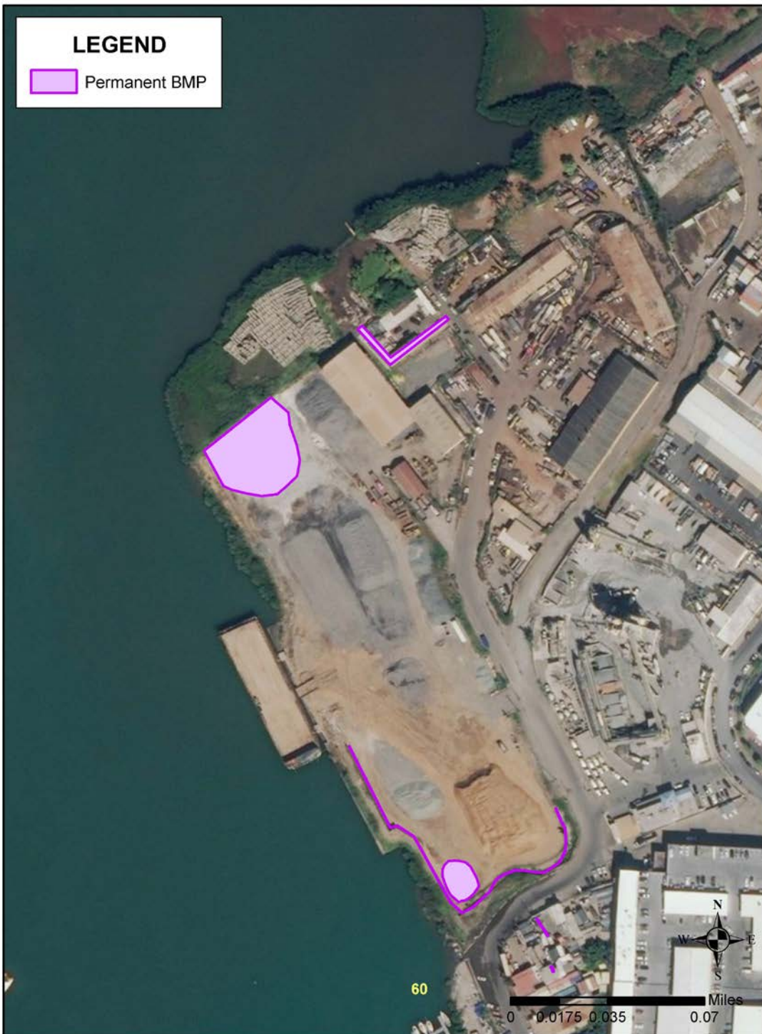
Figure 12C. Honolulu Harbor Post-Construction BMPs with GIS map of BMP locations.
