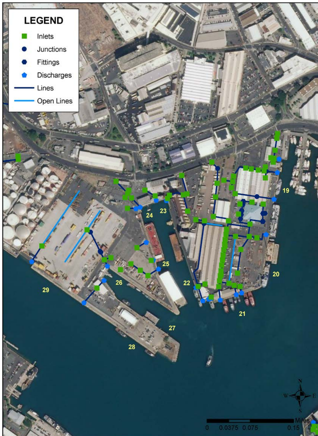
Figure 7. Piers 19 through 29 GIS map of storm drain assets.
