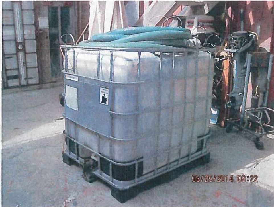
Photo 9: One 250-gallon IBC used to store sanitary wastewater temporarily (facing southwest). Contractor pumps out the waste on a regular schedule.
