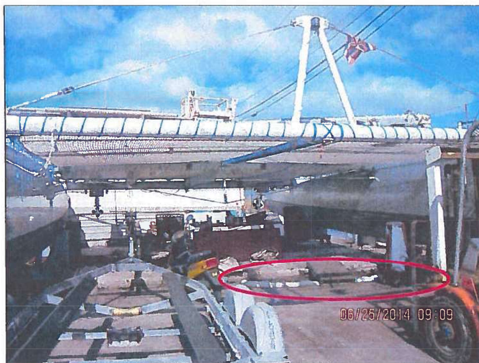
Photo 4: One catamaran on-site to be repaired (facing west-southwest). Beneath the vessel is the trench drain bermed with biosocks (circled in red).
