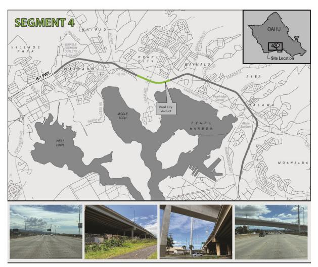
**Segment 4 – Pearl City Viaduct:** This section of the freeway is elevated on piers. A total of six (6) lanes including the HOV lane on the left and the AM Peak lane on the right are carried through this segment. The Pearl Harbor Bike Path is located approximately 30 feet makai of the current edge of the viaduct, at ground level. A portion of the viaduct is within the Special Management Area (SMA).
