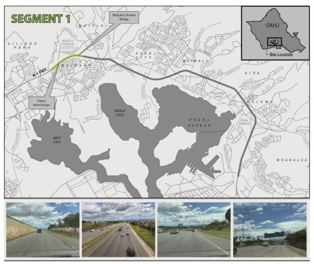
**Segment 1 – Paiwa Street to Waiawa Interchange:** This section of the freeway is mostly at ground level. Raised sections include the Paiwa Street Overpass and the Waipahu Stream Bridge. The main feature of this segment is the close proximity of residential properties along the makai edge of the right of way.
