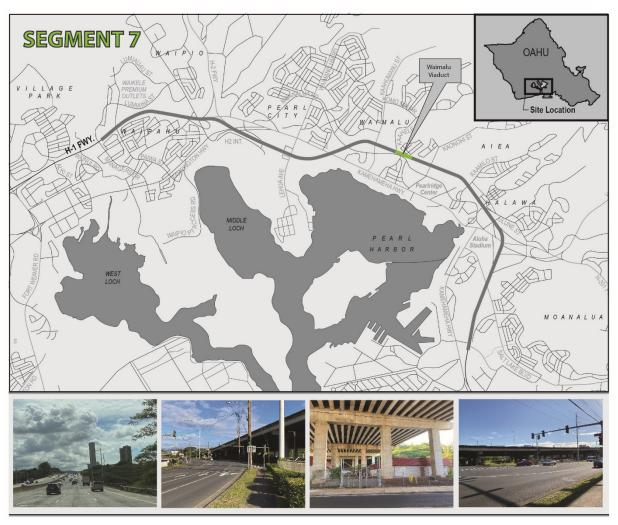
**Segment 7 - Waimalu Viaduct**: At the Waimalu Viaduct, the freeway is elevated on piers. The viaduct crosses over the Waimalu Stream. A curving section of the City and County of Honolulu owned Moanalua Road is located immediately adjacent to the edge of the existing viaduct. Utilities, including those strung along utility poles, occur in close proximity to the elevated freeway deck.
