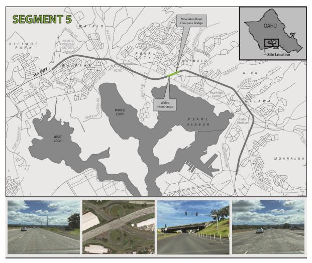
**Segment 5 – Waiau Interchange**: The Waiau interchange provides access to and from Moanalua Road. The interchange includes tight radius on- and off-ramps in close proximity to each other. In the eastbound direction, the right lane and AM Peak shoulder lane are merged into one off-ramp lane, leaving five (5) lanes continuing on. Two eastbound on-ramp lanes from Moanalua Road are carried across the Moanalua Road Overpass bridge. During non-peak hours
