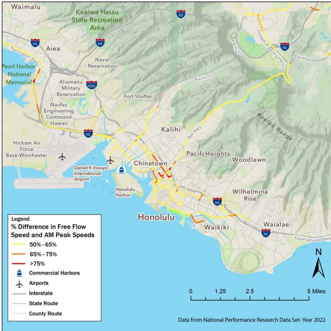
Figure 3-20 Truck Bottleneck Locations with 50% or Greater Difference in Free Flow Speeds and AM Peak Speeds – Honolulu, Oahu
