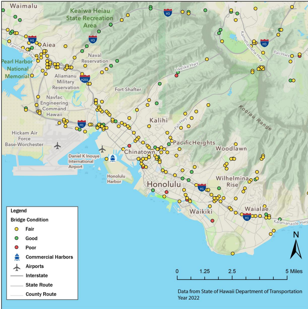
Figure 3-42 Overall Bridge Condition - Honolulu, Oahu
