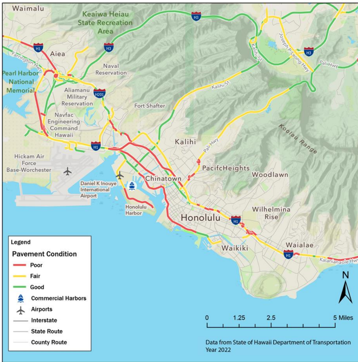
Figure 3-37 Overall Pavement Condition - Honolulu, Oahu
