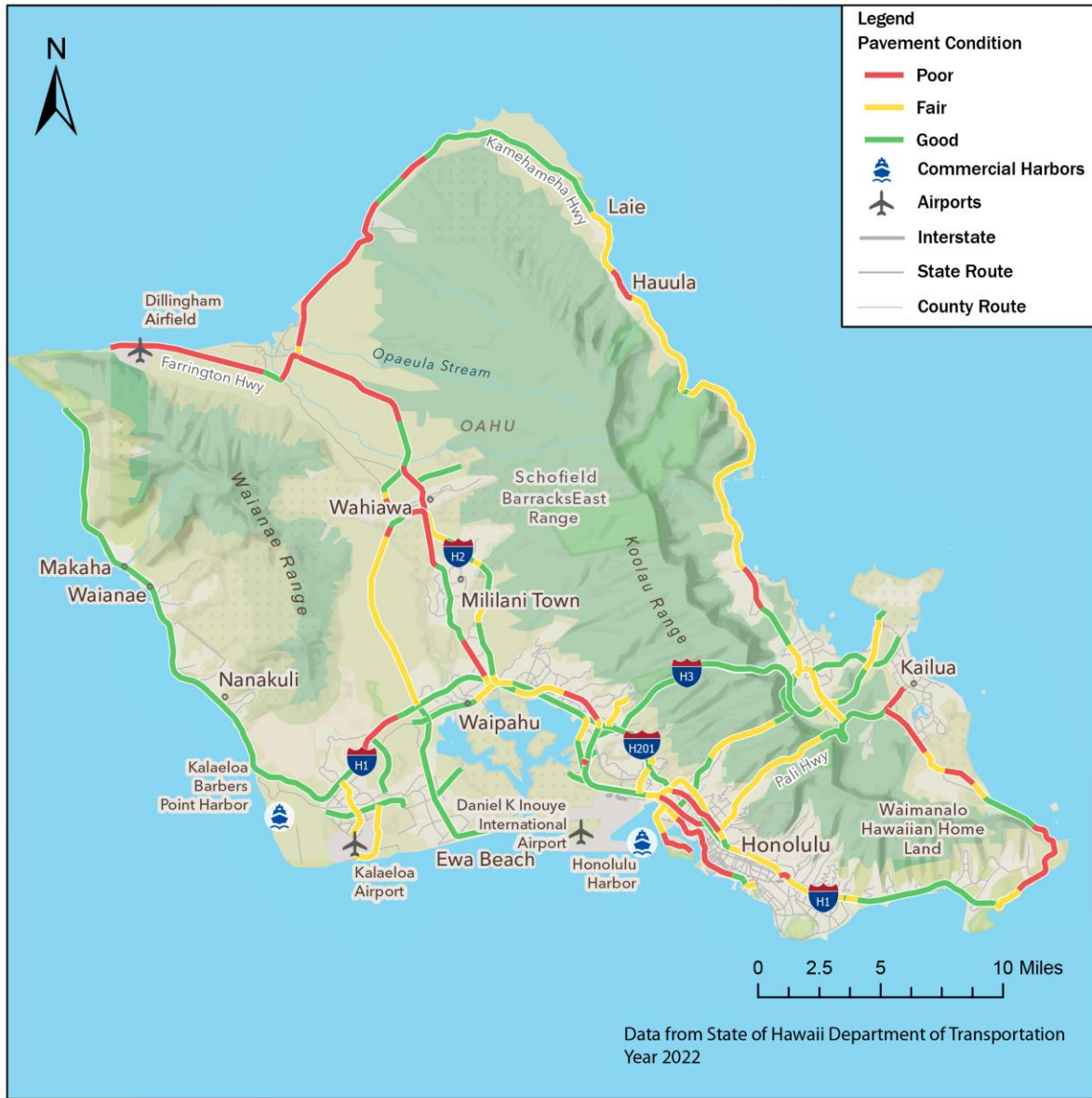
Figure 3-36 Overall Pavement Condition - Oahu
