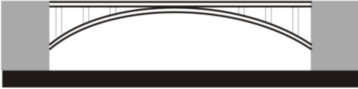
FIGURE 13. OPEN SPANDREL ARCH BRIDGE (PARSONS BRINCKERHOFF, A CONTEXT FOR COMMON HISTORIC BRIDGE TYPES, 3-68).
