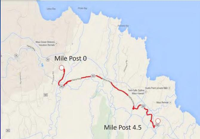
SCOPE Cold planing, resurface existing pavement, pavement markings & signage, reconstruct weakened pavement areas
