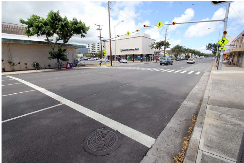
Example 7: King Street at Hauoli Street: Pedestrian activated mast arm flashing beacons.
