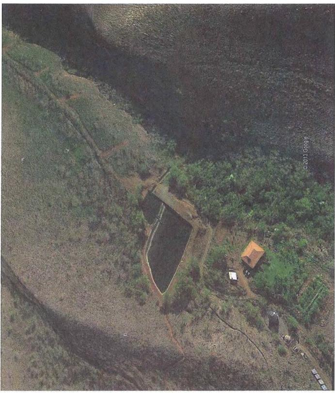
Figure 10. Launiupoko Reservoirs showing Launiupoko Ditch that brings water down from the stream intake to the smaller sediment collection pond. Excess waters can overflow back into the stream, although this rarely if ever occurs. Reservoir water is then distributed downslope for irrigation.
