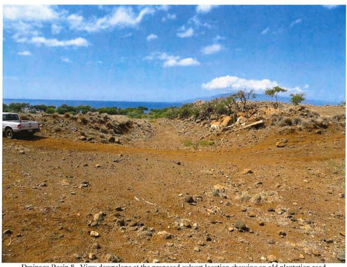
Drainage Basin 8. View downslope at the proposed culvert location showing an old plantation road alongside a pile of field stones. There is a slight swale but no identifiable channel is visible. Sheet flow from local rainfall encounters a six foot high berm above the cane haul road that prevents water from reaching the highway or the ocean.
