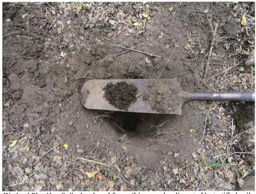
Wetland Plot 1b – Soils developed from silting pond sediment. Unstratified soils included dry silt from 0-38 inches and Loamy Silt from 38 to 54 inches.
